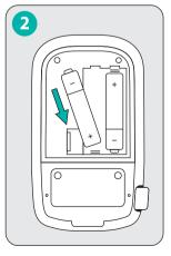
Place the batteries, remember about the correct polarity + -.
