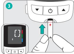
Insert a test strip. You will hear the beep sound and moving lines will appear on the screen.
