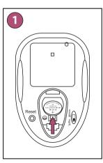
Place the batteries, remember about the correct polarity + -.
