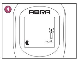
A flashing ♠ means that the device is ready to take a blood sample. Use M button to mark a test as pre-meal ♠ or post-meal ♠.
