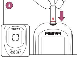
Insert a test strip. You will hear the beep sound and moving lines will appear on the display.
